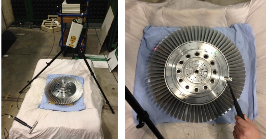
Figure 2: Impact hammer – (Left) Test setup with laser vibrometer, (Right) Excitation with roving hammer
